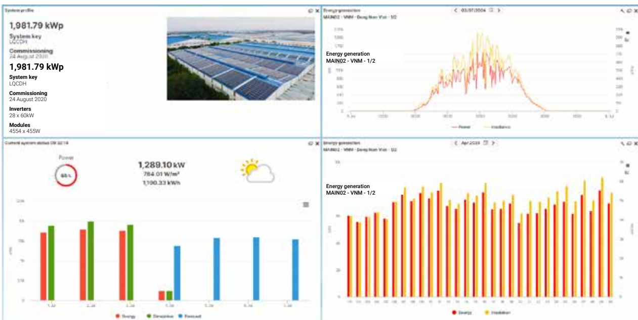
Figure 20: The power and output of a RTS system are tracked through the monitoring system
