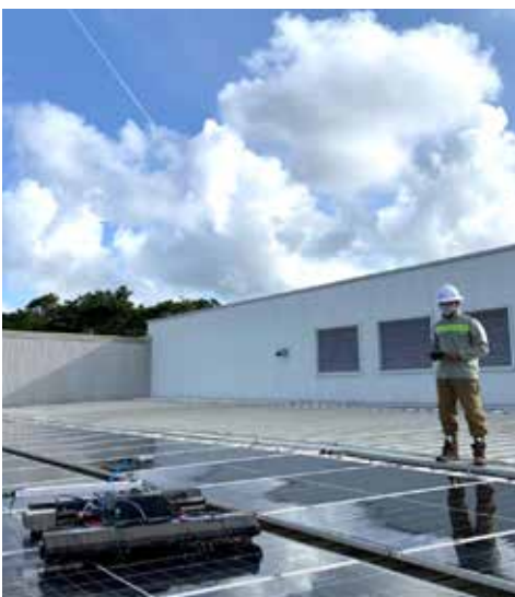
Figure 28: Using robots to clean PV panels
