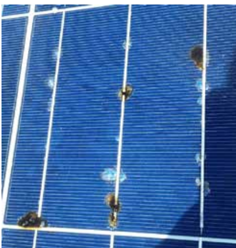
Figure 32: PV panel shaded by trees and hotspot phenomenon
